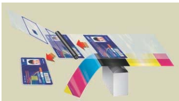
Re-Transfer printing process
