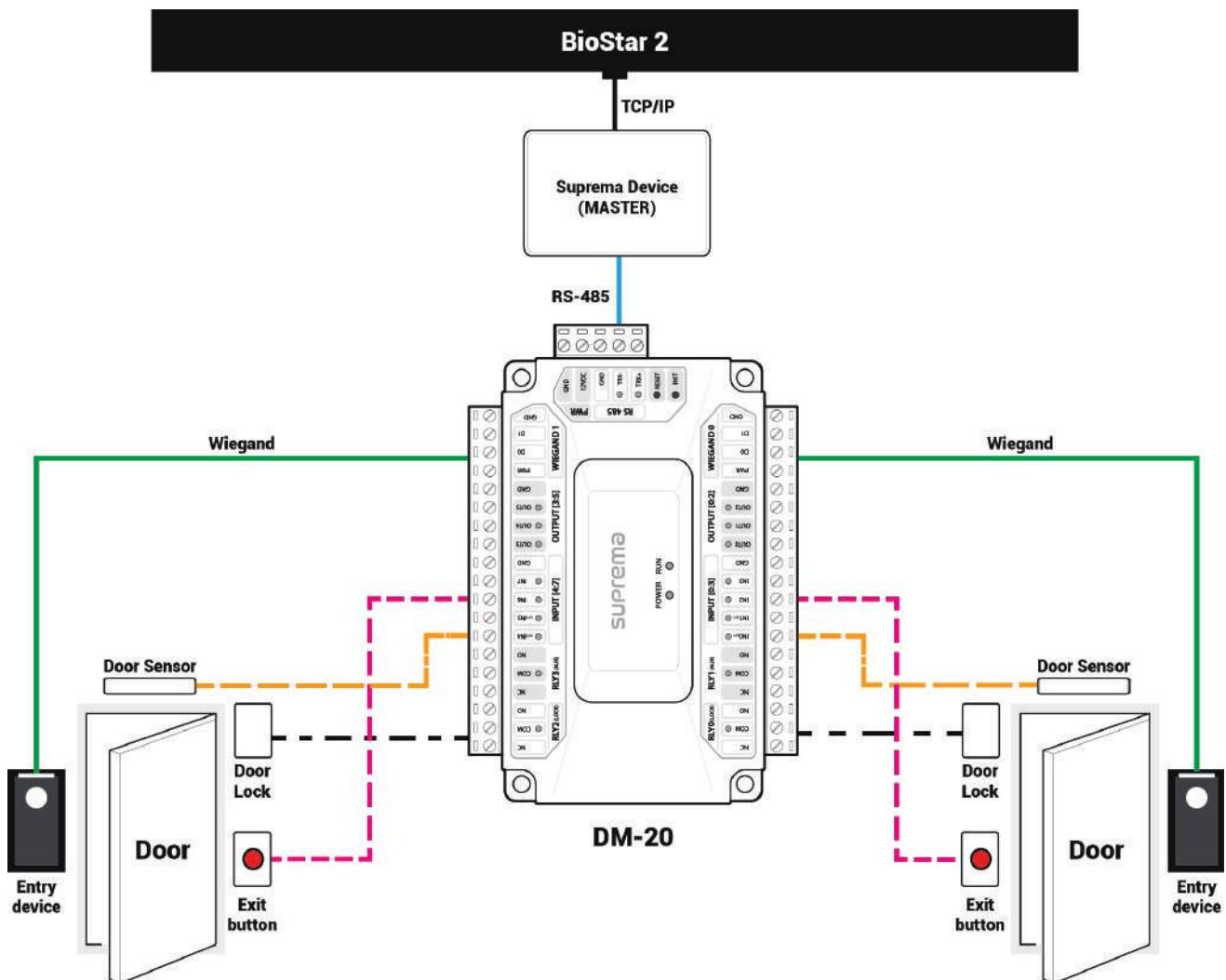
**Components:** Master Device x 1, DM-20 x 1, Suprema Device(Slave) x 1, Wiegand x 2
