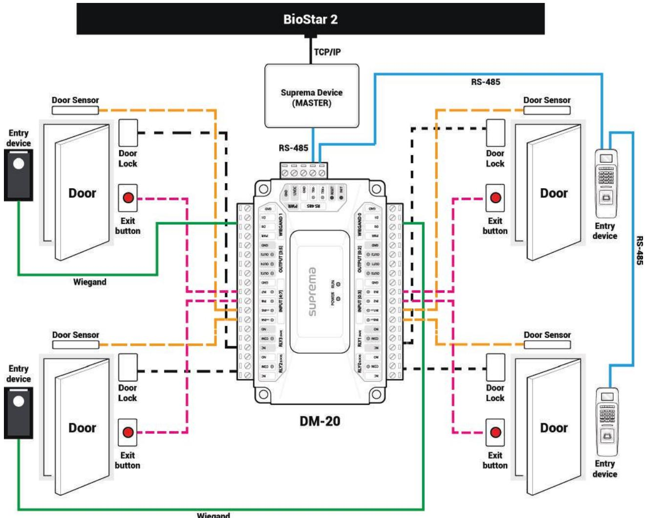
**Components:** Master Device x 1, DM-20 x 2, Wiegand Reader x 4
