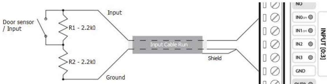
[Example of Supervised Input connection diagram]
